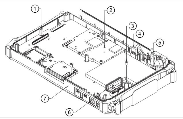
Figure 5-4. Motherboard and LCD Assembly in Top Case
