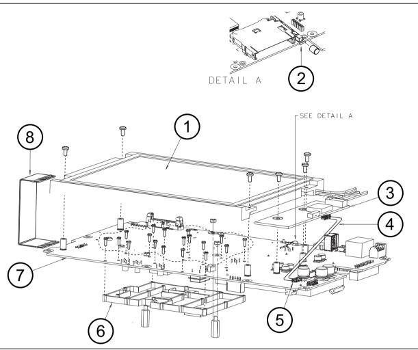
Figure 5-5. Motherboard and LCD Display
