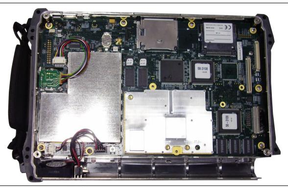
Figure 5-10. Removing the Main PCB
