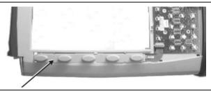
Figure 5-16. Function Hard Key Membrane and Switchpad
