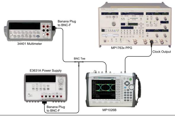
Figure 3-2. Amplitude Accuracy Test Setup
