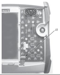
Figure 5-15. Connector J2 on Keypad PCB
