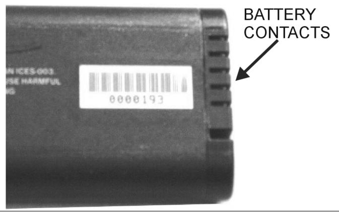
Figure 4-5. Battery Contacts
