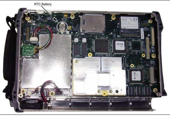
Figure 5-9. RTC Battery Location
