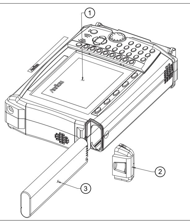
Figure 5-1. Bit Master Case and Parts Overview
