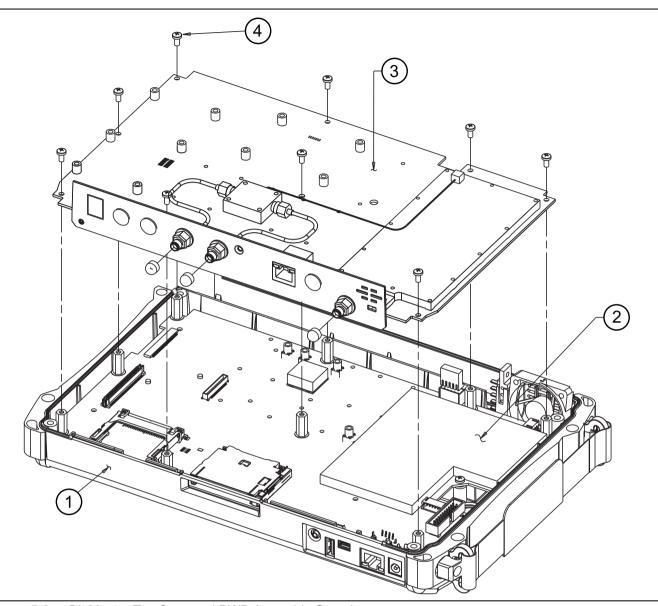
Figure 5-3. Bit Master Top Case and PWB Assembly Overview
