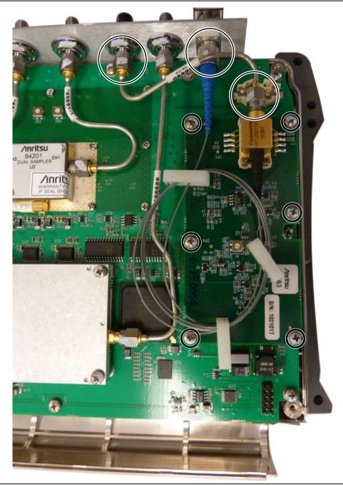
Figure 5-13. Optical/Electrical Module Removal
