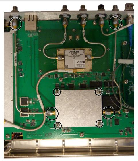
Figure 5-12. Clock Recovery Unit Module Removal
