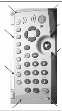
Figure 5-14. Locking Tabs on Front Bezel
