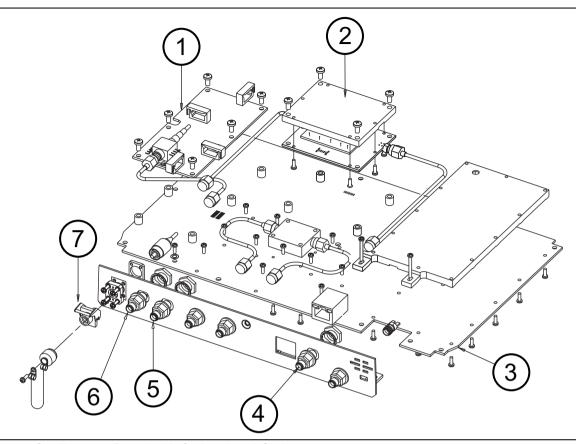
Figure 5-7. Oscilloscope Board with Option 2 and Option 3
