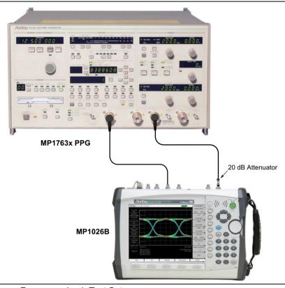
Figure 2-1. Clock Trigger Frequency Lock Test Setup
