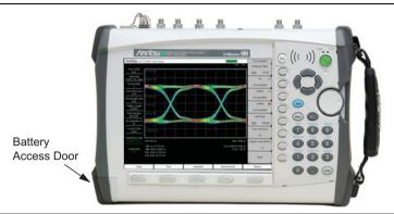
Figure 4-1. MP1026 Battery Access Door Location
