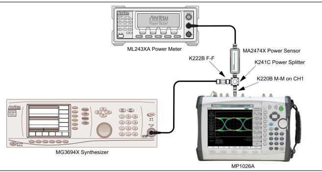
Figure 3-1. Bandwidth Verification Setup
